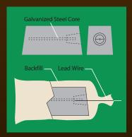
Packaged Anodes are prepackaged in a cardboard carton in low resistivity, quick wetting prepared backfill consisting of 75% hydrated gypsum, 20% bentonite, and 5% sodium sulfate.
